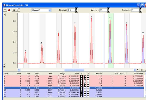
Peaks automatically detected and displayed in Flow Analysis window
